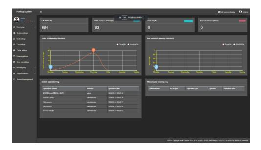
2.2 The online monitoring page can monitor the vehicles entering and leaving the parking lot in real time, and can remotely open the gate for abnormal vehicles.
